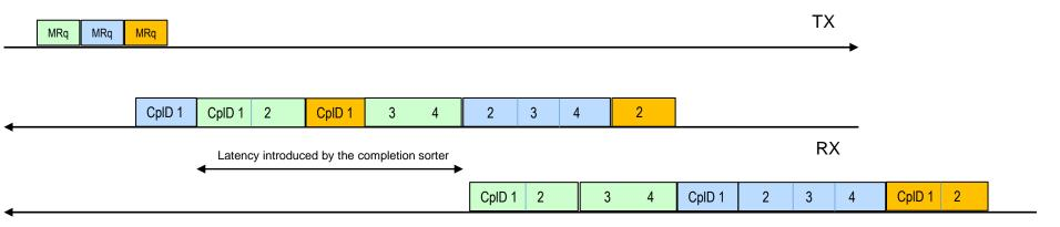
Sorted sequence in the FPGA after completion sorting
